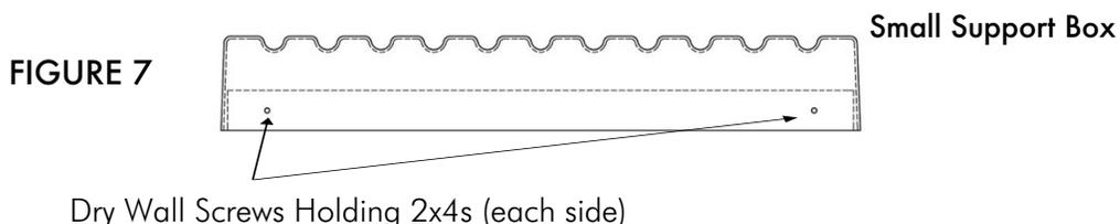
4. Insert the small box in the channel. At this point, do not adhere the small support box to anything. Place the large support box into the channel and over the top of the small box. Place the CleanCut Convertible into position and compress downward to determine the proper height and placement for the support box structure.
