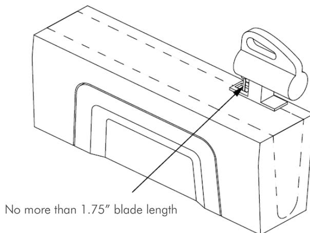
8. It is required that proper eye protection be worn while using the jigsaw. Cut the bottom of the CleanCut Convertible using the jigsaw cutting directly on the center of the traced lines. Upon reaching the corners while cutting, tilt the jigsaw outward to prevent cutting past your lines on the vertical ends of the CleanCut Convertible. Remember to tilt your blade on each corner. On the ends of the CleanCut Convertible, simply continue the cutting process with the jigsaw.
